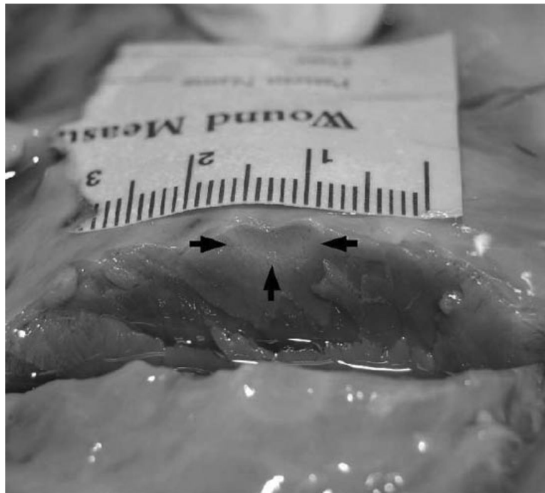
Fig. 4. Cross section of ablation site in bovine cardiac tissue. The black arrows indicate the approximate distal and lateral boundaries of the ablated region; centimeters are numbered in the presented scale.
