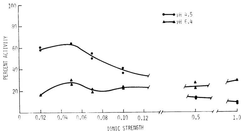
FIG. 5. Effect of ionic strength on the percentage activity remaining in solution after 8 min of heating at 70 C. Initial concentration was 100  $\mu\text{g}/\text{ml}$ .
