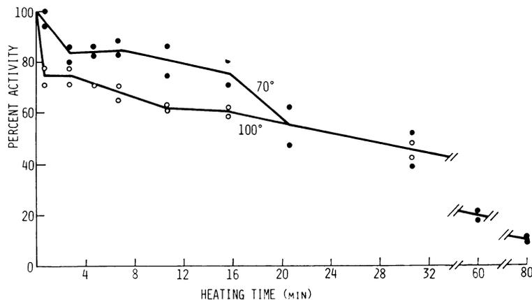
FIG. 6. Heat inactivation of enterotoxin B at pH 4.5. Initial concentration, 100  $\mu\text{g}/\text{ml}$ ; ionic strength, 0.02.
