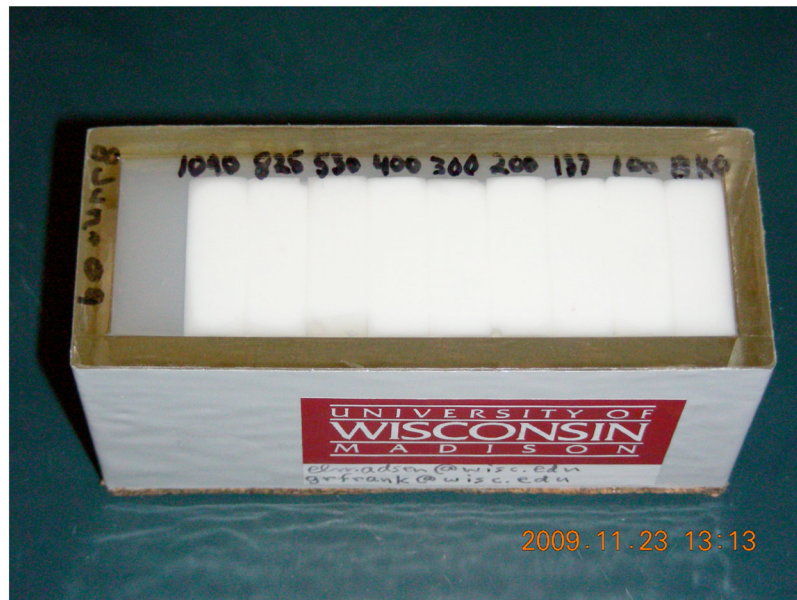
Fig. 2. Photograph of phantom 2. The nine 3\text{cm} \times 3\text{cm} \times 1\text{cm} blocks are seen through the Saran Wrap® scanning window.
