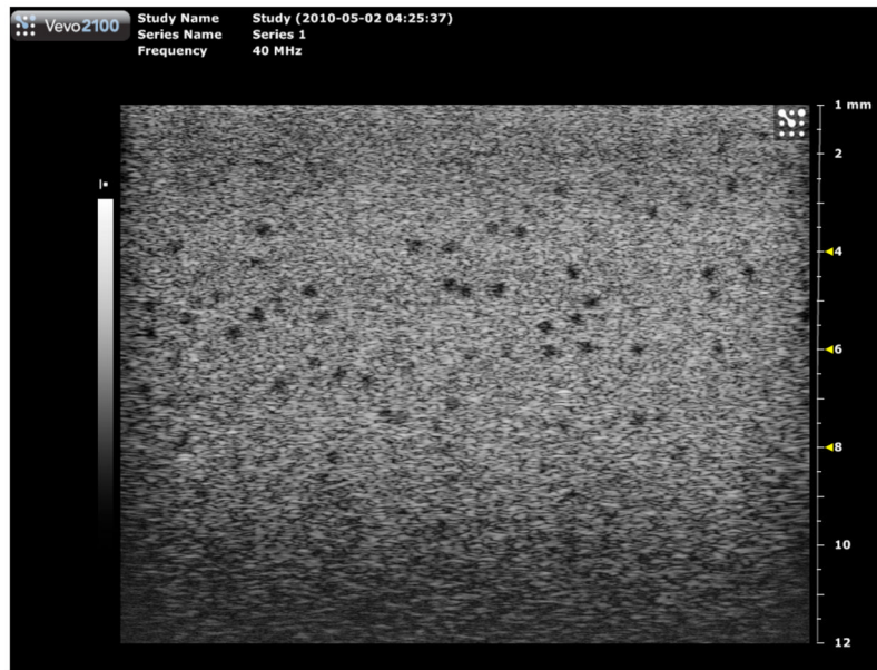
Fig. 10. Image of the section of phantom 2 containing 290- \mu\text{m} diameter anechoic spheres using the Vevo 2100 40 MHz model 550 linear array transducer. Multiple focuses at 4, 6 and 8 mm were used corresponding to the results shown in Figure 14. Note that this image was made at a little greater field of view than those used in generating Fig. 15.
