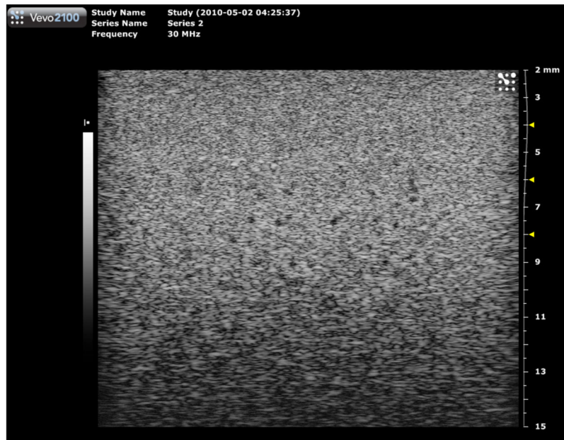
Fig. 11. Image of the section of phantom 2 containing 290- \mu\text{m} diameter anechoic spheres using the Vevo 2100 30 MHz model 400 linear array transducer. Multiple focuses at 4, 6 and 8 mm were used corresponding to the results shown in Figures 13 and 14. Note that this image was made at a little greater field of view than those used in generating Figs. 14 and 15.
