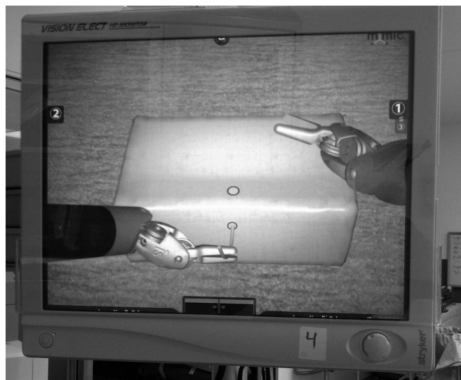
Figure 4. Screen shot of da Vinci Skills Simulator “suture sponge level 1” needle-driving exercise.
