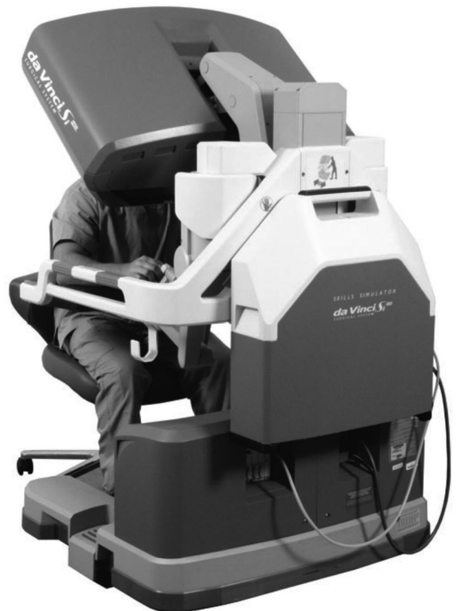
Figure 1. da Vinci Skills Simulator shown attached to da Vinci Surgical Si console. 17
