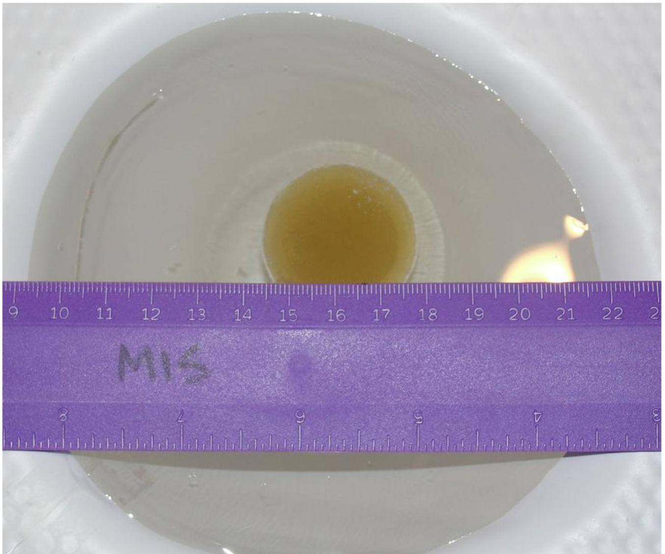
Figure 5. The spherical saline gel target inclusion suspended in the plastic breast model
