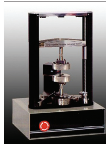
Figure 3: Apparatus for measuring the sample toughness
