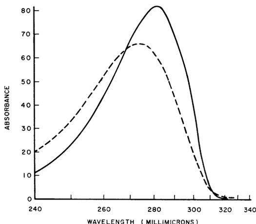
FIG. 2. UV spectra of DMMA. Symbols: dashed line, *cis,cis* configuration; solid line, *trans,trans* configuration.
