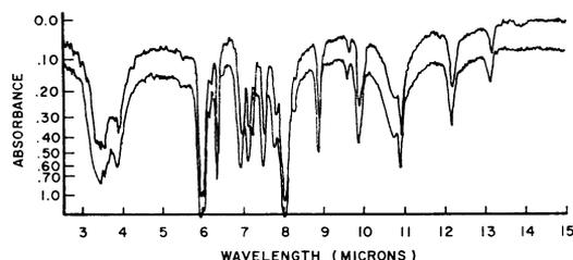
FIG. 1. Infrared spectra of synthetic (upper scan) and biologically prepared (lower scan) DMMA (*cis,cis* isomers).
