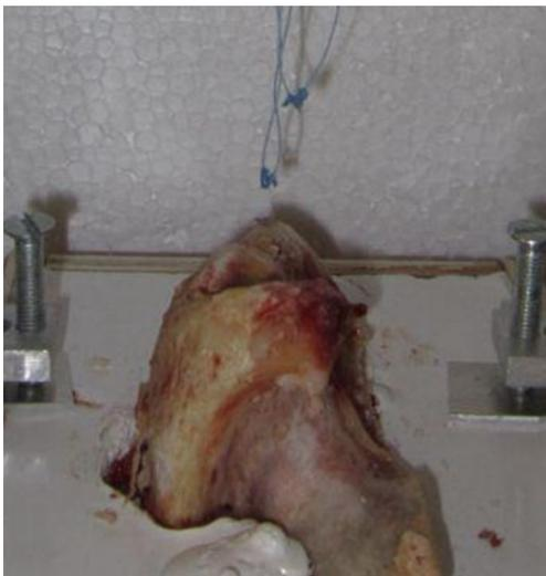
**Fig. 4** All suture anchor (ASA) failure: anchor detachment
