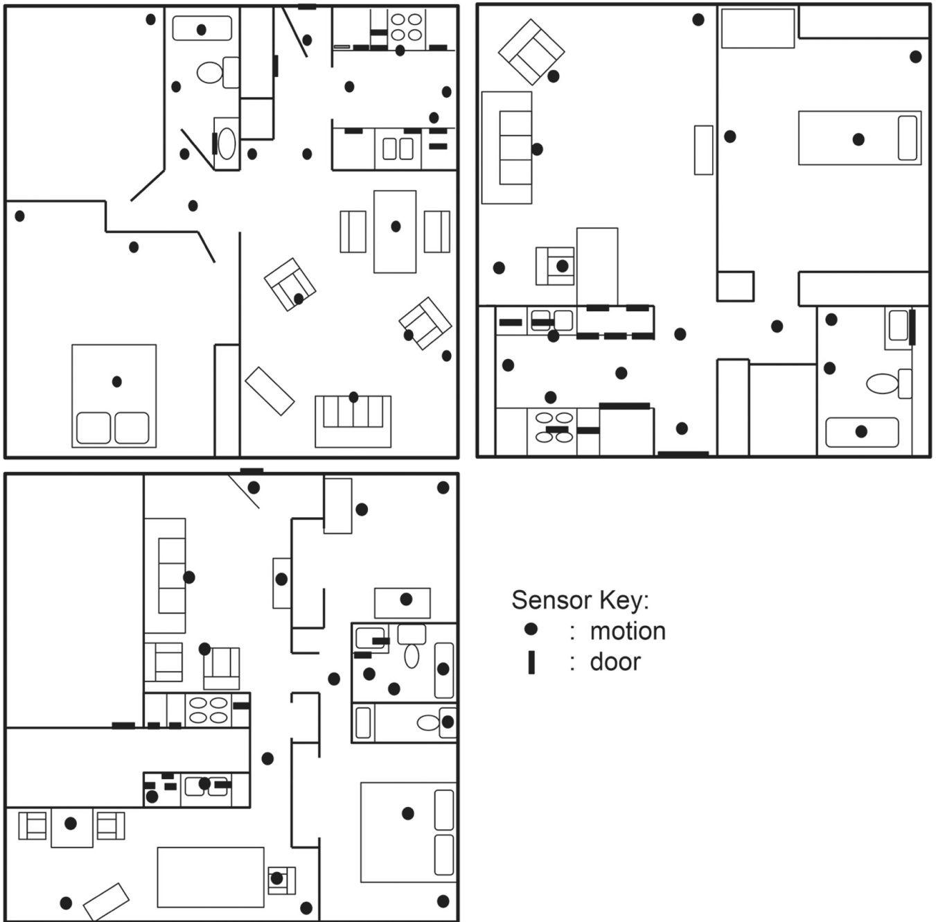
Figure 3. The sensor layouts (black circles) and doors (black rectangles) for the three apartments: B1(top left), B2 (top right), and B3 (bottom)
