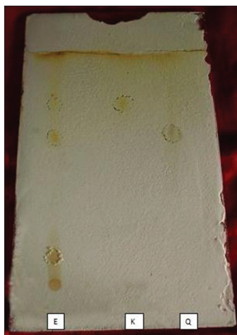
Figure 1: Thin layer chromatography. E: Extract; K: Kaempferol; Q: Quercetin
