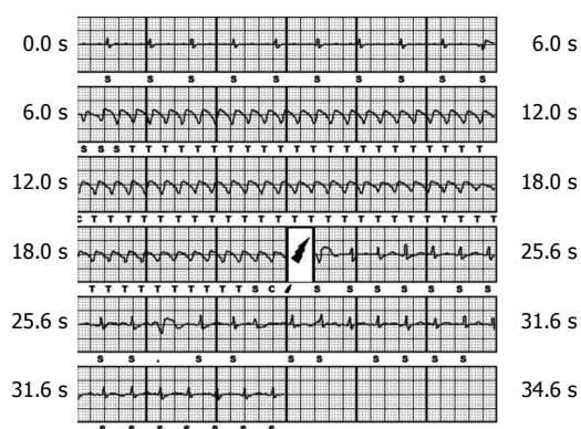
Figure 3 Subcutaneous implantable cardioverter-defibrillator electrogram showing a sustained monomorphic ventricular tachycardia that is terminated by a shock (lightning symbol). The subcutaneous implantable cardioverter-defibrillator (S-ICD) system uses an 18/24 interval criterion for tachycardia detection (T) which is reconfirmed after capacitor charging (C), but before shock delivery, to exclude the presence of non-sustained tachyarrhythmias. S: Sensed event not classified as tachycardia.
