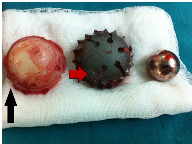
Fig. 3. The picture shows the polyethylene wear at the edge of the liner (black arrow) and the crack pattern in the shell (red arrow).
