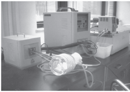
Figure 1. Portable inductive heating device and water jacket incubator.
