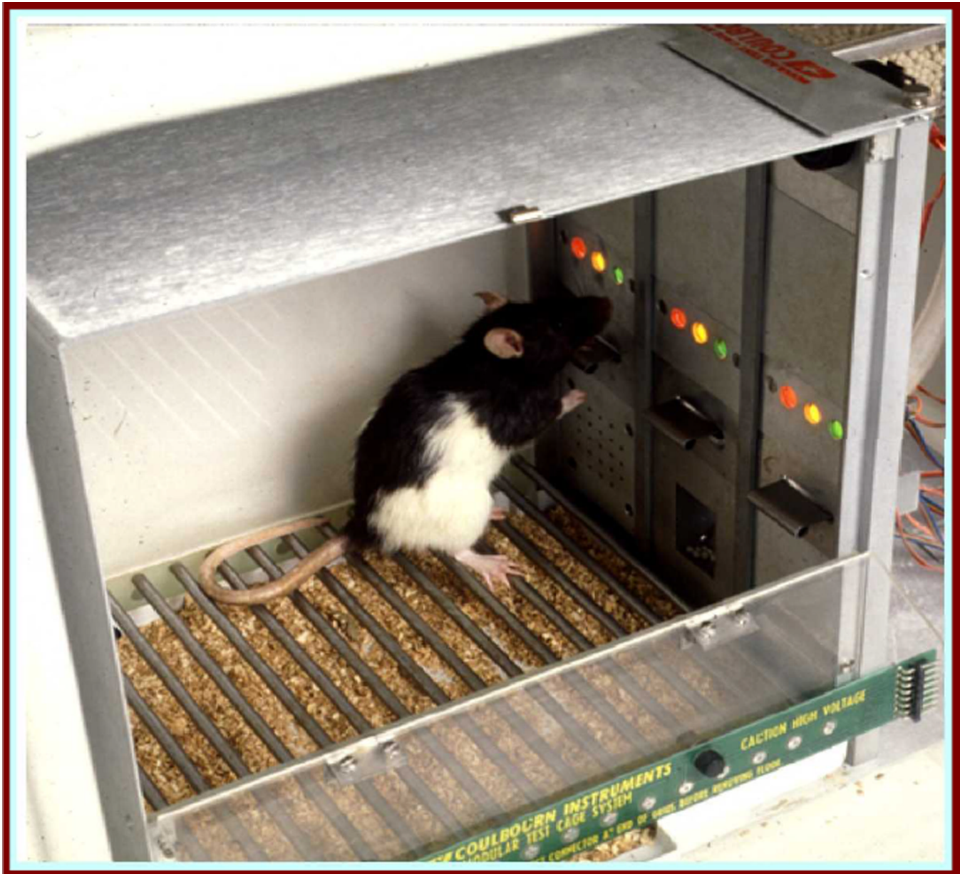
Figure 1. Standard operant chamber containing response levers, feeder (behind panel), and stimulus lights
