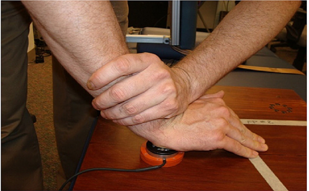
Fig. 1. A photograph showing the force transducer, force plate, and the doctor's hand position for delivering simulated HVLA thrusts. (Color version of figure is available online.)
