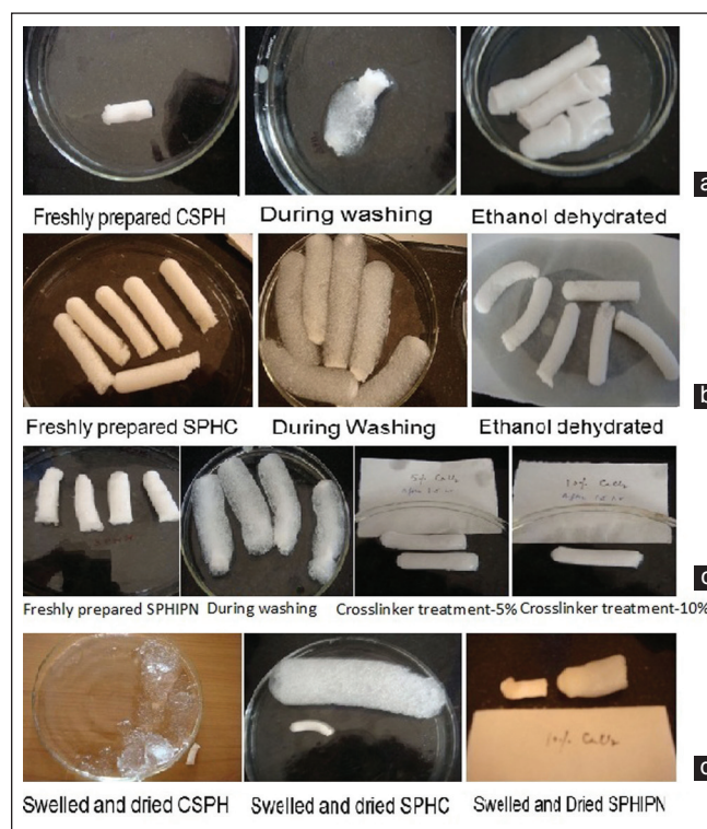
Figure 1: Various steps during synthesis of different generation superporous hydrogel (a) conventional superporous hydrogel (CSPH), (b) superporous hydrogel composites (c) superporous hydrogel interpenetrating networks (SPHIPNs), (d) swelled and dried CSPH, SPHC and SPHIPN
