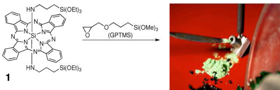
Figure 2. Bis -amino Si phthalocyanine 1 derivative was formed initially. Its reaction with GPTMS resulted in a Si phthalocyanine sol-gel glass that was ground and sieved to 150 \mu\text{m} -sized particles, of which 35 mg quantity was loaded into the device.
