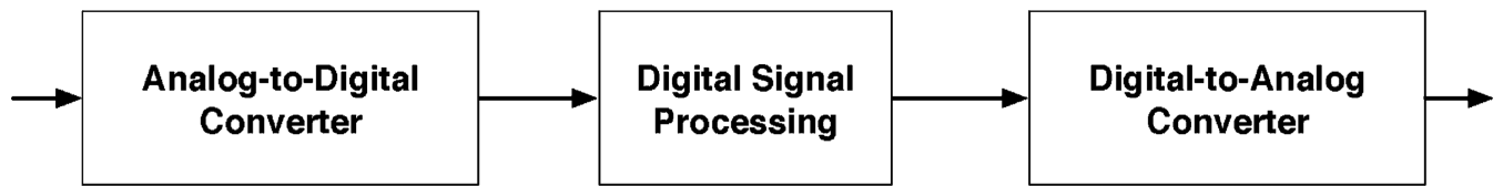
Fig. 1. General signal processing chain with a digital signal processing core.
