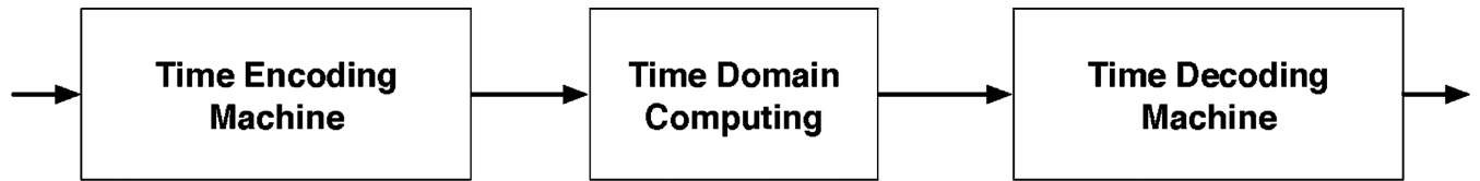
Fig. 2. General signal processing chain with a time domain computing core.
