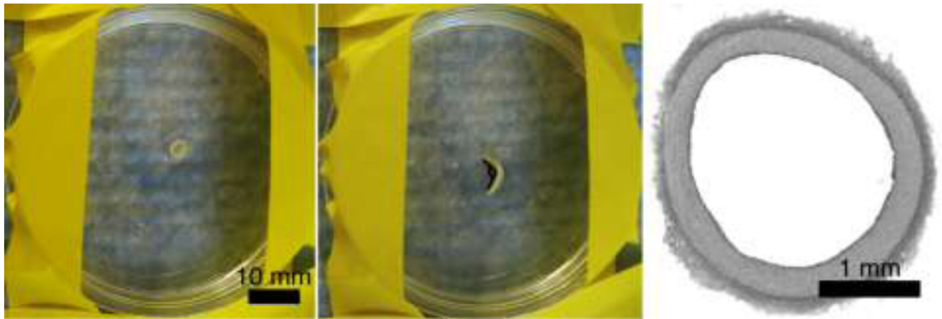
Figure 1. Representative opening angle demonstration of a proximal porcine coronary artery. Left: vessel before splaying. Middle: vessel section after splaying with representative angle measurement markers. Right: Histology image to get vessel dimensions (hematoxylin and eosin stain).
