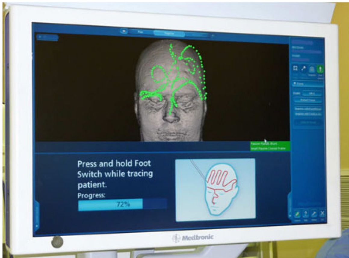
Fig. 1. Standard display from the StealthStation (Medtronic Inc., Minneapolis, MN) neurosurgical guidance system. The green points represent the data acquired from a tracked pointer, superimposed on the patient's skull generated from preoperative images. The red points demonstrate point selection for the user.
