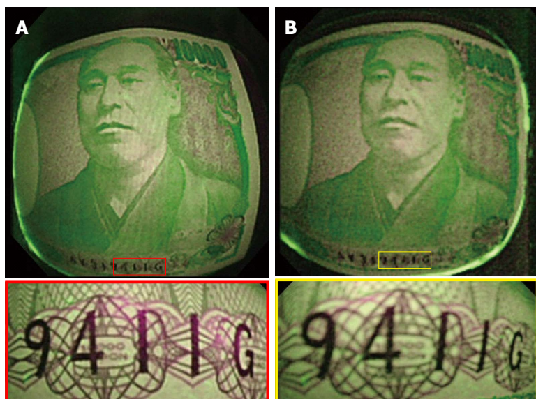
Figure 1 Comparisons of images obtained with the previous autofluorescence imaging system and with the novel autofluorescence imaging system. The major improvement in the novel autofluorescence imaging (AFI) system is in the image-processing algorithm, specifically the noise-reduction algorithm, which results in higher resolution images with less noise interference. An AFI image from the previous AFI system (A: EVIS LUSERA ERITE CLV-290) is clearer than an image from the novel AFI system (B: EVIS LUSERA CLV-260).
