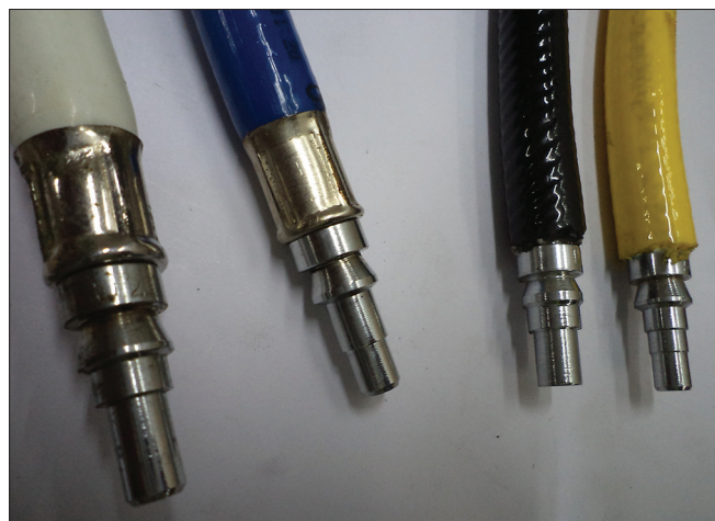
Figure 6: Schraeder probes for different gases
