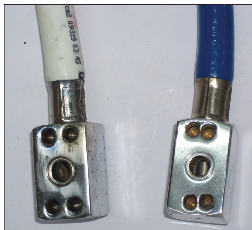
Figure 7: Non-interchangeable screw threaded connection for different gases
