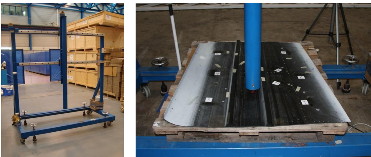
Figure 3. Certified impact machine to be used with aeronautical specimens.
