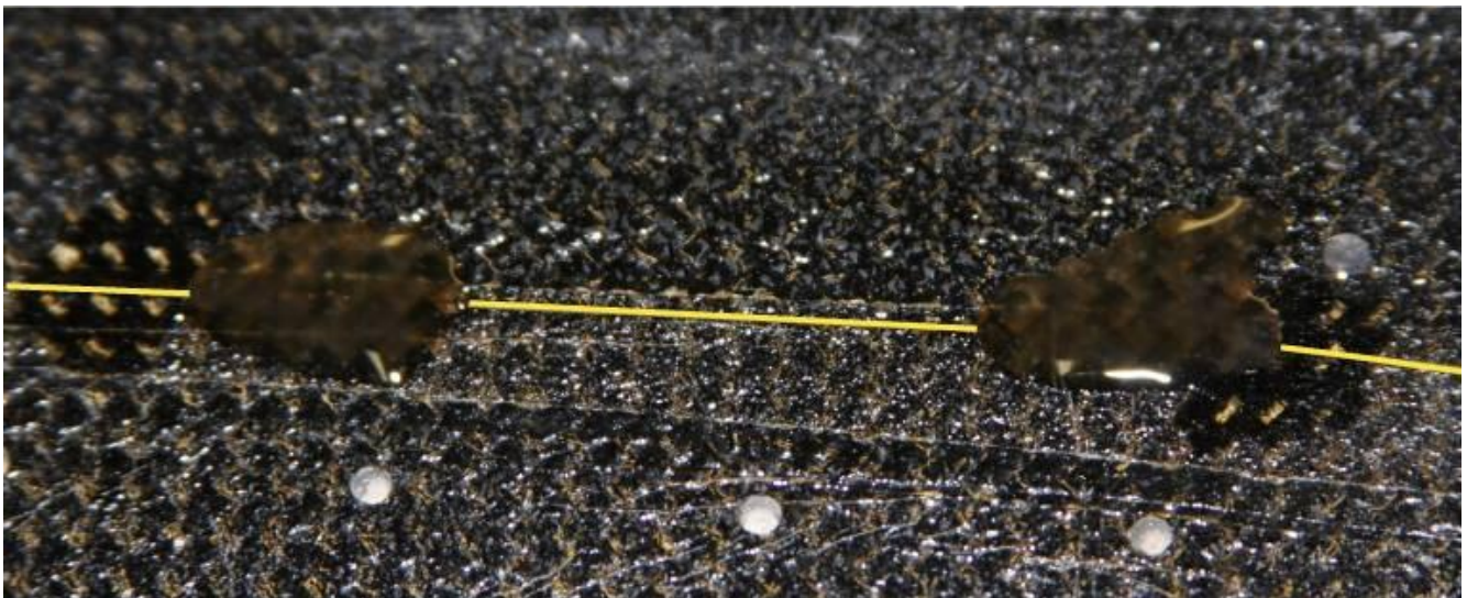
Figure 2. Detail of an installed Fiber Bragg Grating using epoxy as bond material.
