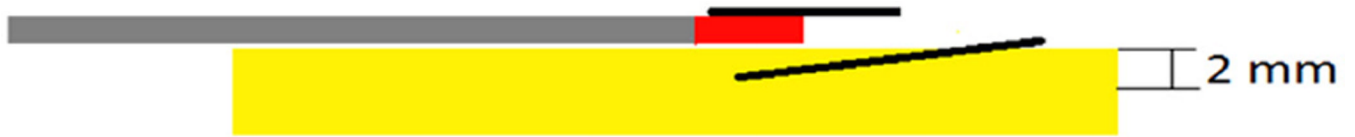
Figure 6. Heating schematic for phantom disk. The catheter (gray) is positioned close to the surface of the tissue-mimicking phantom (yellow) with the transducer elements (red) centered on the thermocouple needle (black). Note also a thermocouple needle (black line) on the backside of the transducer elements.
