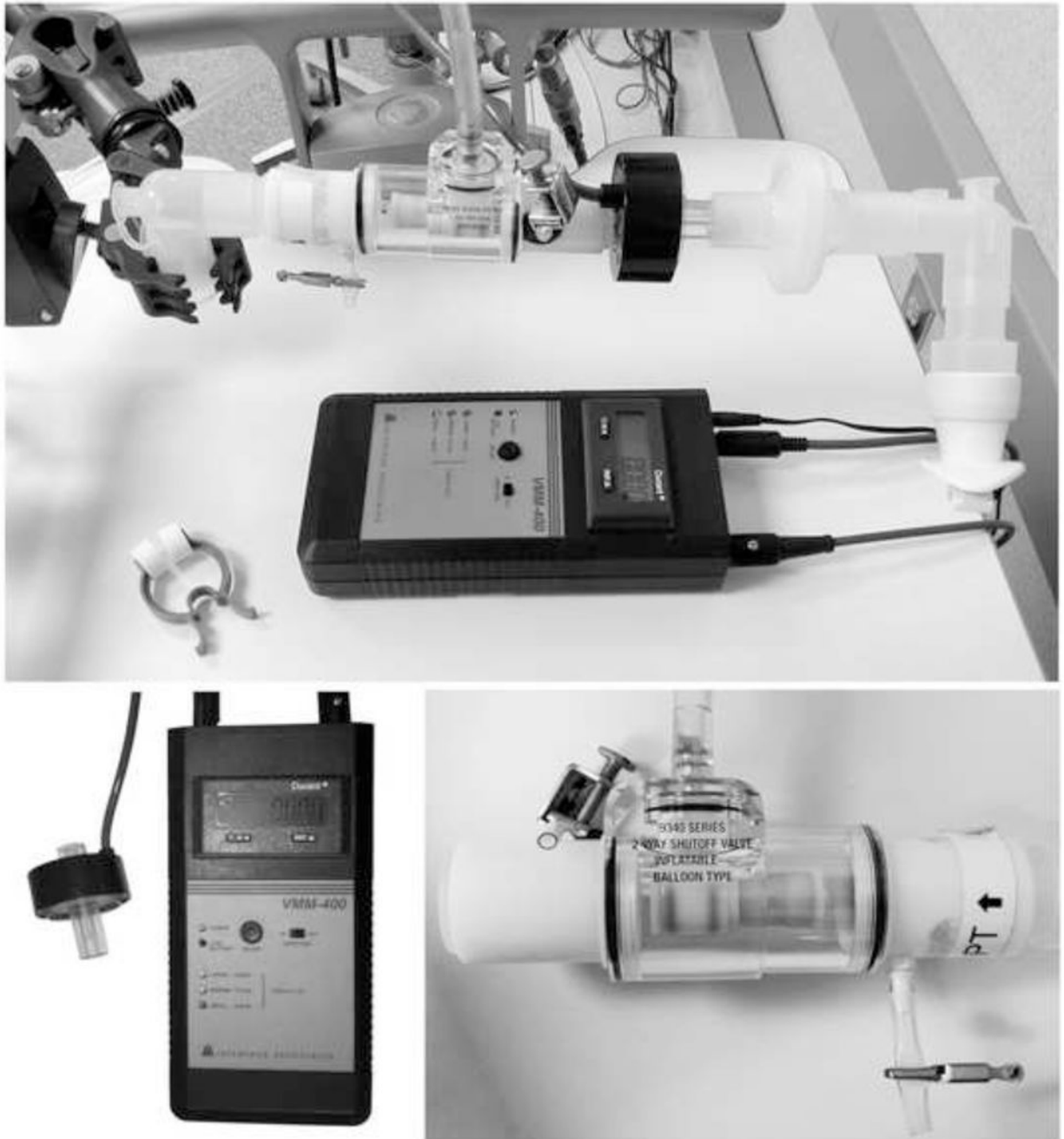
Figure 1. Components of the turbine-based breath-hold lung volume controller: overall system ( top panel ); Interface USA, VMM-400 turbine-based flow meter ( bottom-left panel ); Hans Rudolph two-way balloon occlusion valve ( bottom-right panel ).
