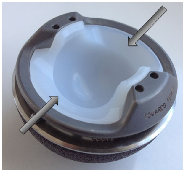
Fig. 1 The TLC liner. Note the cutouts on either side of the retaining fingers that accommodate the neck during internal and external rotation, both in flexion and extension, if properly aligned. Adjacent fingers or prongs supported by a metal ring prevent the fingers from spreading and allowing the head to escape.
