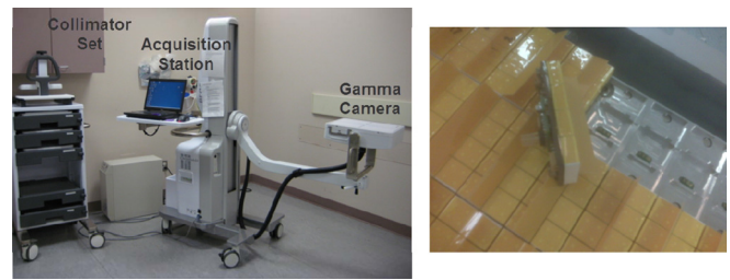
Fig. 1. (Left) The Ergo system pictured here shows the gamma camera on an arm extension, a laptop acquisition station, and a collimator shelf with several different collimators. (Right) The image shows the details of the detector consisting of modules of the indirect CsI coupled with Si photodiodes that are mounted on an electronic readout board.
