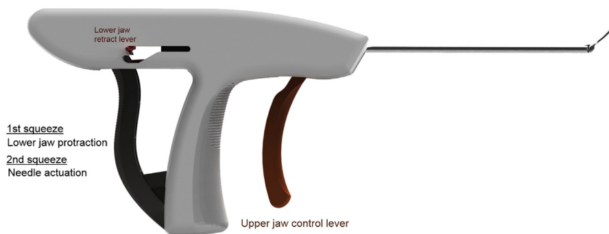
Fig 2. Profile view of Ceterix meniscus suture passer. The orange trigger controls the upper jaw; when compressed, the upper jaw flexes forward so that it can be brought in line with the shaft during insertion into the knee. The black trigger has dual functionality: lower jaw protraction and needle drive. When compressed the first time, the lower jaw protracts forward, and when compressed a second time, the needle passes the suture from the lower jaw to the upper jaw, where it is self retained. The lower jaw can then be retracted back into the shaft by use of downward pressure on the thumb trigger so that the device can be atraumatically removed. The device is designed for use with 1 hand. The surgeon can place multiple stitches with 1 disposable device.
