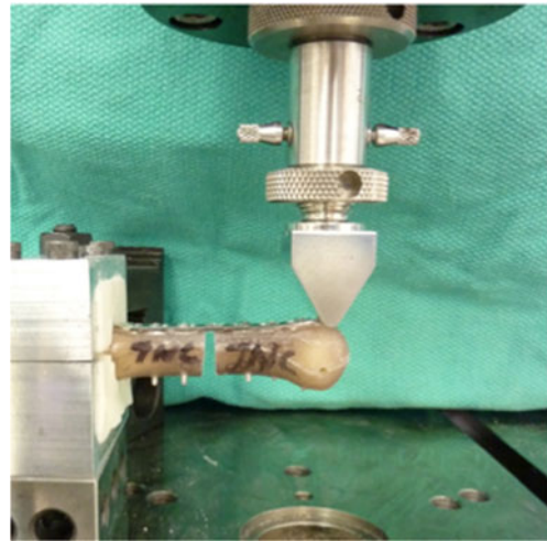
Fig. 1 Setup for cantilever bending testing. The specimen represents a locking construct with four cortices of fixation per segment
