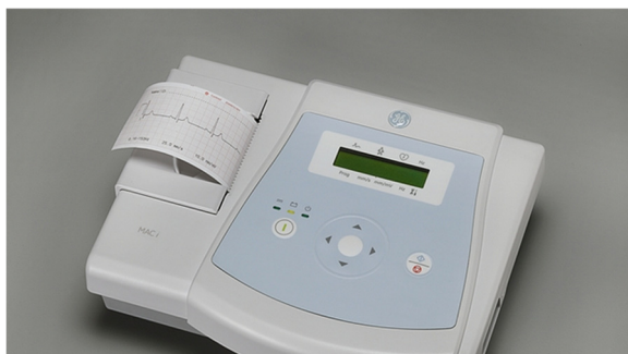
Figure 3 General electric MACi ECG machine [7].
