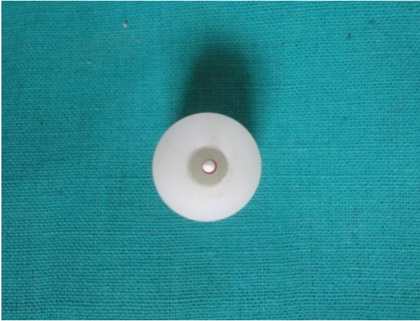
Fig. 1: Plastic mould with post positioned perpendicularly in the centre.
