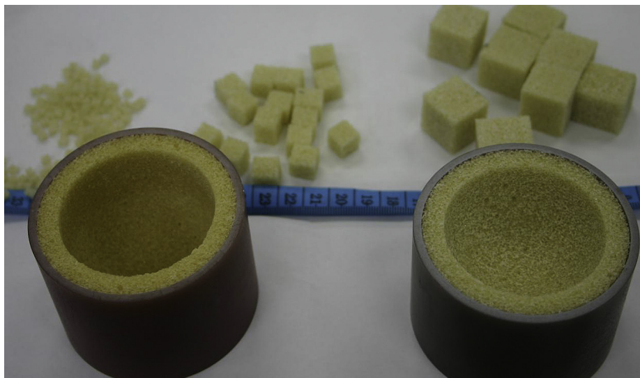
Fig. 1 – Two acetabular models with sawbone graft in background. The acetabular model on the right in the figure is from the control group with a 53 mm spherical central defect to 26 mm depth. The acetabular model on the left is taken prior to impaction grafting of the protrusio defect of depth 46 mm.
