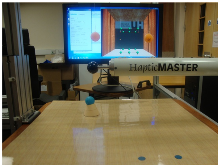
Figure 2 Virtual environment set-up. Green balls represented source and target points for various segments. An inflating target ball plus an audio cue was used to start movement for each segment. Red and grey cylinders, shown in Figure 3, appeared as the movement progressed from source to target.
