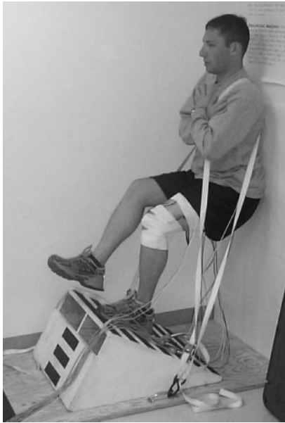
Figure 2. Measurements for a closed kinetic chain maximum voluntary isometric contraction were collected and used to normalize all electromyographic data.
