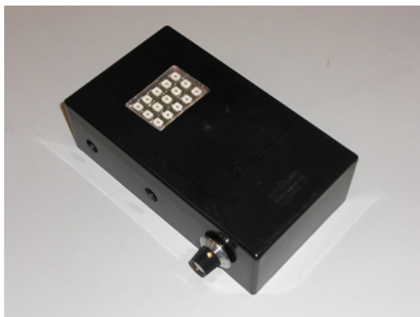
Fig. 7. LED array device for in vitro experiments
