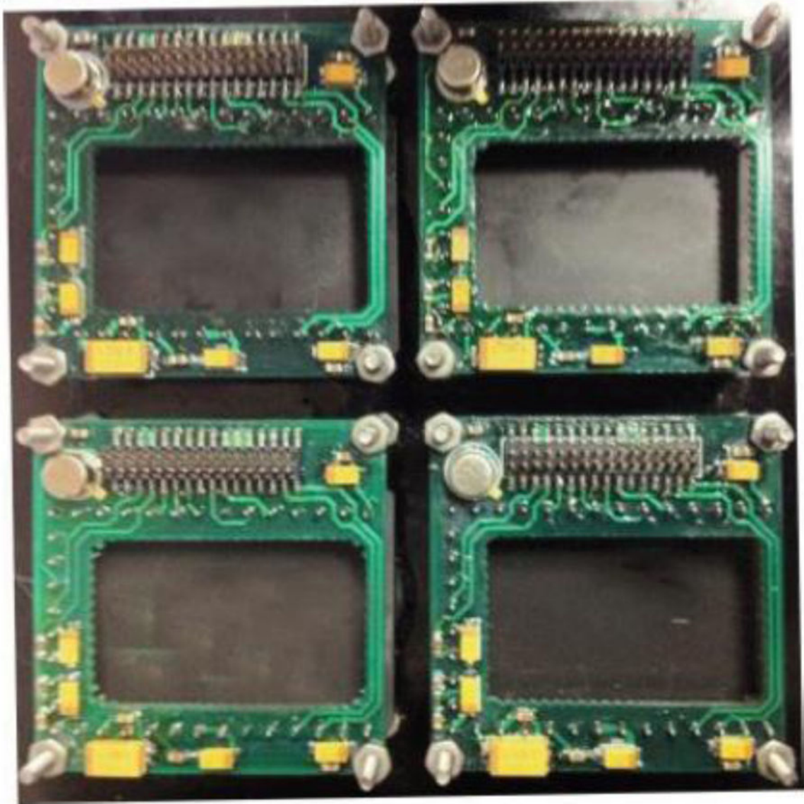
Figure 4. Rear view of a 2×2 assembly of the headboards, with sensors mounted on the front.
