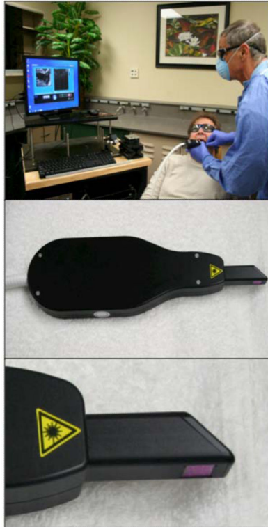
Fig. 1. Photographs of the 3D CP-OCT scanner showing the scanning handpiece along with the 6×6 mm scanning window at the end of the scanner.
