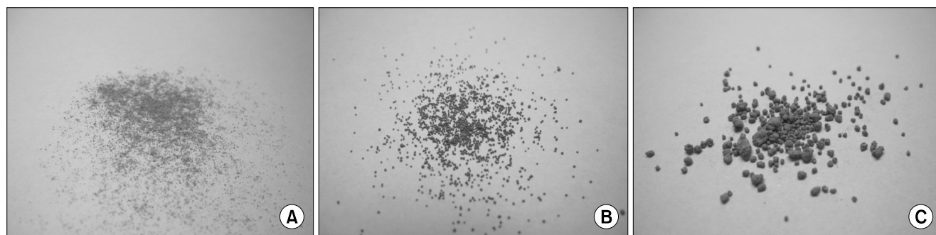
Fig. 1. Images showing the measured particle sizes of saltwort powder granules obtained with the fluidized bed coater. (A) Less than 0.2 mm, (B) 0.2~0.6 mm, (C) larger than 0.6 mm.
