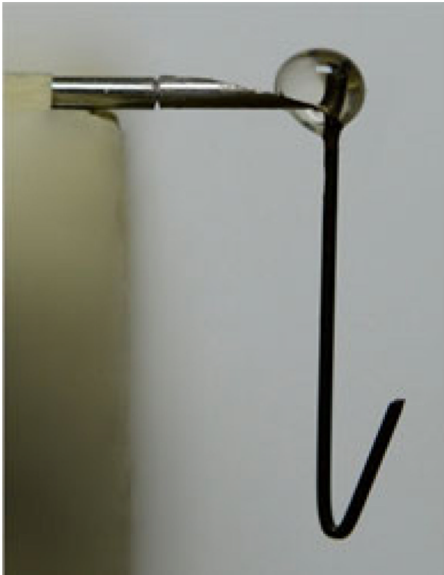
Fig. 2. Experimental flexure stiffness test setup.
