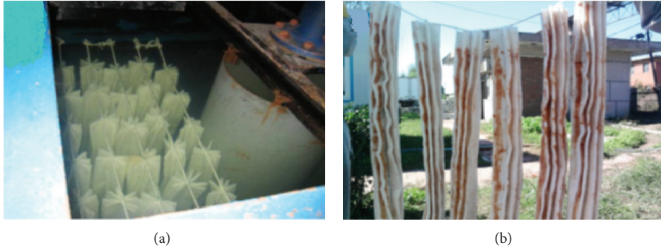
FIGURE 8: Images of the pilot-scale ANAMMOX reactor (a) and packing materials (b) [117].
