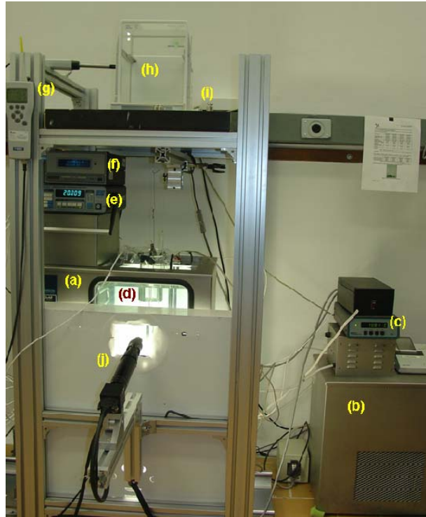
Figure 1. Hydrometer Calibration System: (a) thermostatic bath; (b) external cooler; (c) external temperature controller; (d) glass vessel containing the reference liquid; (e) thermometer for measuring the liquid temperature; (f) barometer; (g) thermo-hygrometer; (h) weighing instrument (balance); (i) mass standards.
