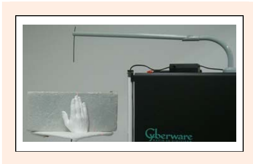
Figure 3. Measurement of hand-model geometry with optical three-dimensional scanner.
