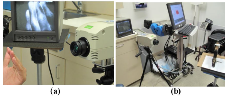
FIGURE 1. (a) THE MERLIN MIDWAVE INFRARED CAMERA AND IMAGE MONITOR AND (b) THE DATA ACQUISITION SETUP USED IN THE EXPERIMENT.
