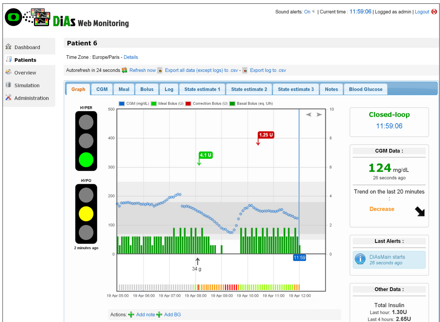
Figure 4. Single patient monitoring screen. Continuous glucose measurements (blue dots) and insulin bolus (green bars) are represented in a chart. Current state of AP, current CGM value and trend, last alerts, and insulin amounts are displayed on the right-hand side. Traffic lights representing hyperglycemia and hypoglycemia risk are on the left-hand side. Other data are accessible from horizontal tabs menu.
