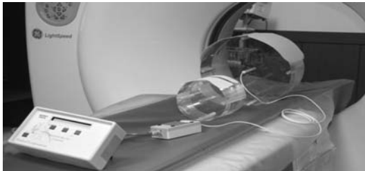
Figure 4. Ionisation chamber, PMMA phantom and bismuth shielding for CT dose measurement.
