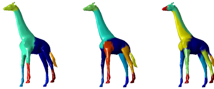
Figure 3. Giraffe shape mesh segmentation with different parameters. A finer scale s detects segments at smaller scales: (left to right) s = 5 , s = 38 , and s = 48 find 8, 10, and 14 segments respectively.
