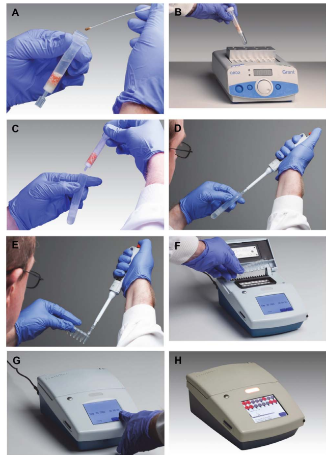
Figure 1. Photographic illustration of the steps of the HE-LAMP-BART. A. Place fecal swab sample into the HE column, mix, seal and twist off the bottom tab of the column; B. Place the column in a collection tube on a hot block at 100^{\circ}\text{C} and incubate for 10 minutes; C. Remove the collection tube and dispose of the column; D&E. Pipette 20 \mu\text{l} of eluate from the collection tube and use this to reconstitute LAMP-BART freeze dried reagent; F&G. Place reconstituted reagent on PDQ and start run; H. Positive results are called in real time. The person in the photograph has given written informed consent, as outlined in the PLOS consent form, to publication of their photograph. doi:10.1371/journal.pone.0083808.g001
