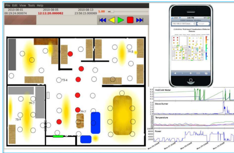
Figure 5. Snapshot of CASAS activity visualizer. The visualizer renders sensor events on a computer or mobile device while plotting usage of resources such as electricity.
