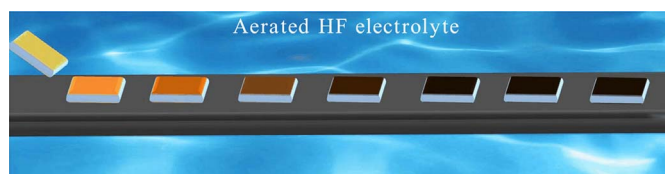
Figure 1 | Schematic overview of continuous production process for SiNWs via substrate-enhanced MCEE of silicon in aerated aqueous HF solution. Silicon substrates coated with noble metal particles are placed in close contact with graphite substrates, and silicon nanowires are produced after passing silicon substrates once through the aerated aqueous HF solution.
