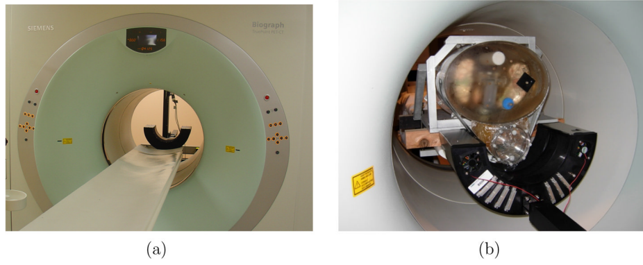
Figure 2. (a) Front View of insert integrated into a Siemens Biograph 40 scanner; (b) Back View of the PET/CT scanner with insert. The chest phantom with custom breast attachment used for the experiments are mounted on the bed with an aluminum holder.
